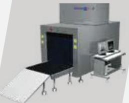
*According to the baggage sizes, these x-ray machines models are different from tunnel size of 60cm x 40cm to 100cm x 120cm. Dual view (Model name with "DV") means the X-ray baggage scanner is designed with 2 x-ray generators, and the x-ray beam shoot from vertical and horizontal directions to scan baggage's and have 2 angles of x-ray images. This technology is upgraded for the improved for international aviation standards.*
